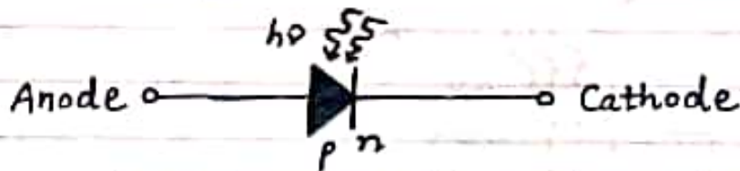
Fig. 1 :- Symbolic representation of a photodiode
